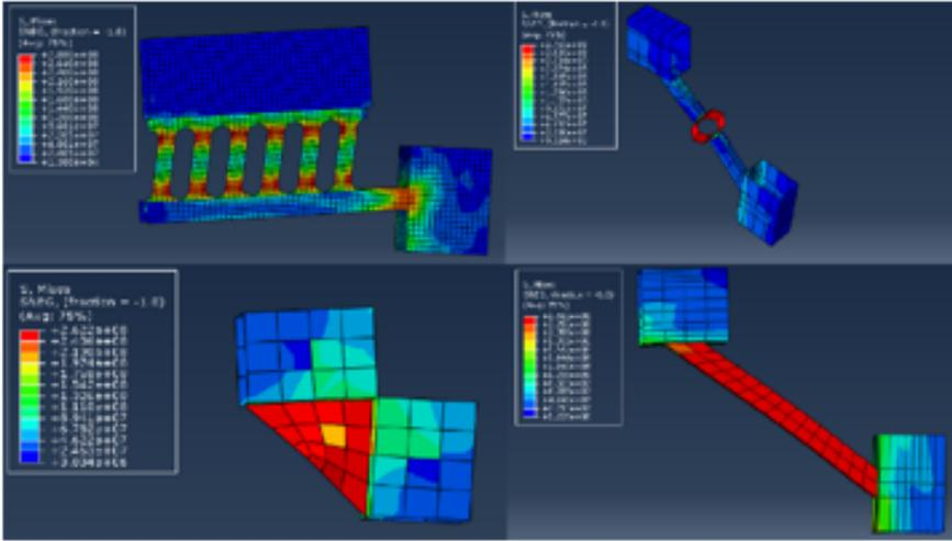
Figure 12: Yielding of reinforcement elements in FD2, FR2, FS2, and FP2
