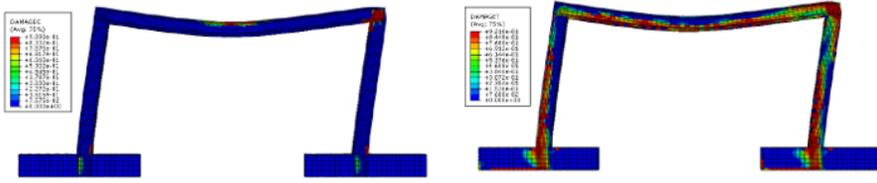
Figure 4: Compressive and tensile damages of ordinary frame
