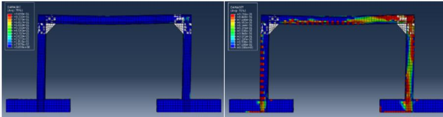
Figure 10: Compressive and tensile damages of FS3 frame
