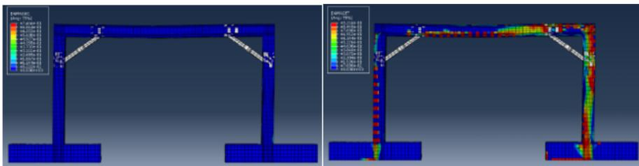
Figure 8: Compressive and tensile damages of FR3 frame
