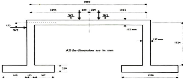
Figure 1: Details of test frame [Cranston and Cracknell \(1969\)](#)
