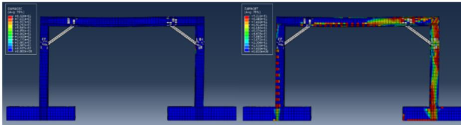
Figure 11: Compressive and tensile damages of FP3 frame
